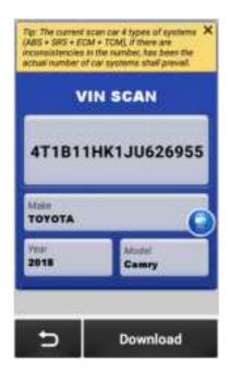
You need to enter the vehicle' s VIN data manually if the MUCAR CDE900 fails to get access to the vehicle VIN data automatically
