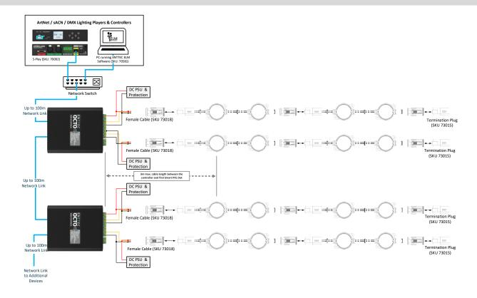
Note: If the power or data source to your controller drops out whilst the Smart PXL Dots remain powered, the last state will be held until either the data feed resumes or power to the Smart PXL Dots is disconnected and re-connected.
