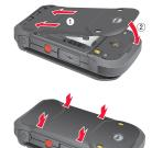
Using a coin, rotate the battery cover screw clockwise until it is tight.
