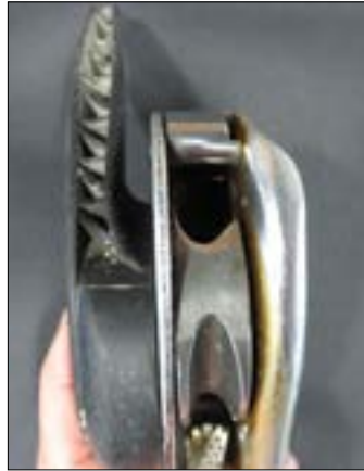
• Worn cam groove
