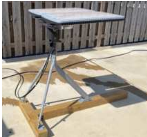
Figure 23: ODU mounted to trimast with mast adapter
