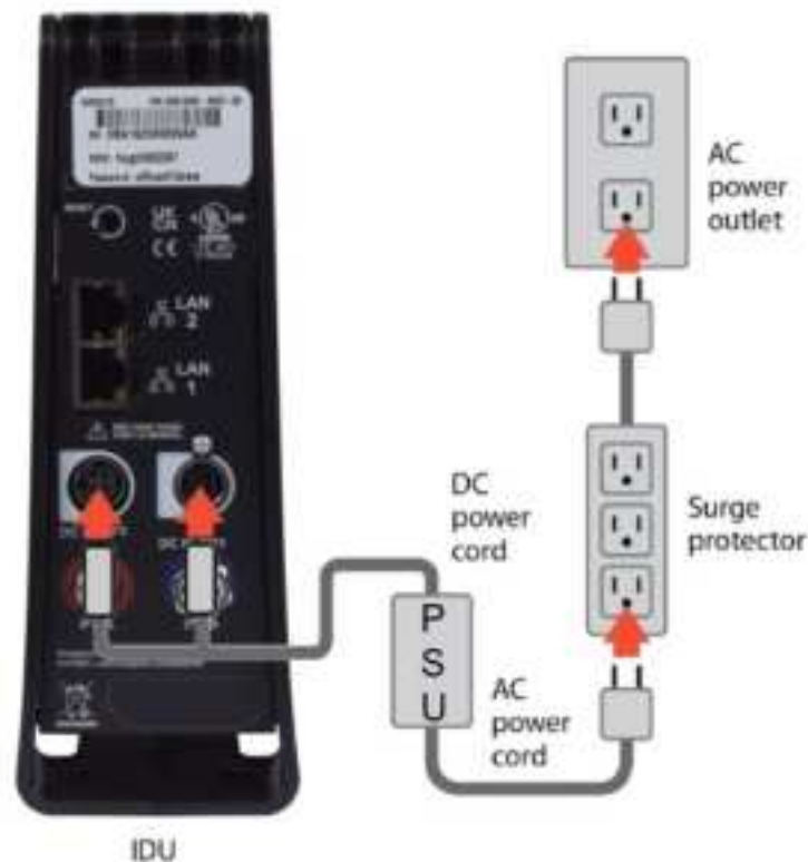
Figure 41: IDU power diagram
