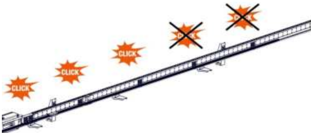
Fig. 37: Do not attach last hanger clamps to additional conductor rails
