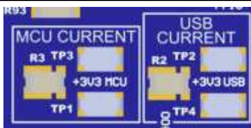
Figure 36. RA MCU and USB Current Measurement
