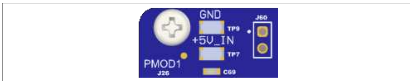
Figure 9. +5 V Test Point Location
