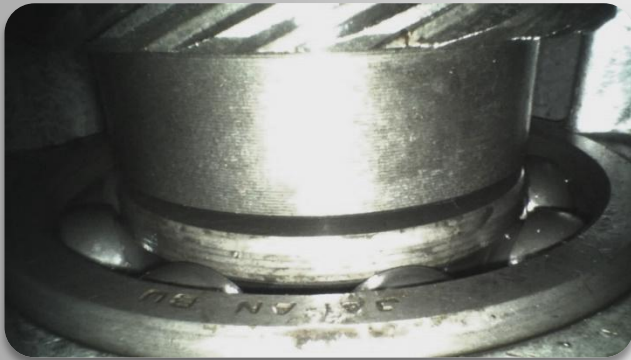
Gearbox Inspection Using a 6mm VQ2 060 1500 4
