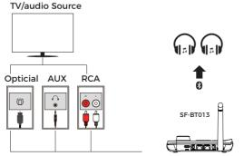
Fig 3: Set up SF-BT013 as Wireless transmitter
