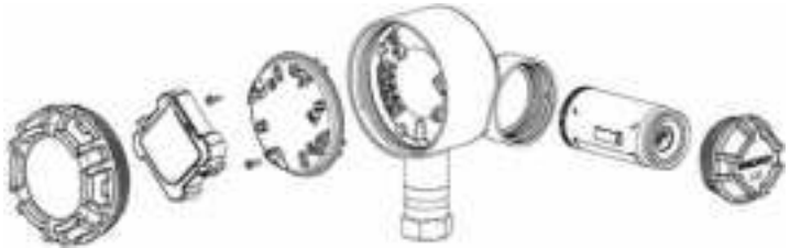
Figure 3-1: Exploded View of LCD Display Assembly
