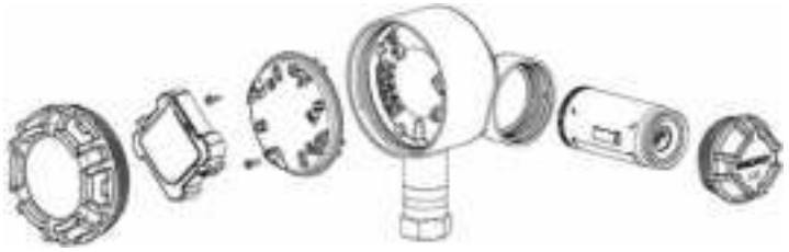
Figure 3-3: Exploded View of LCD Display Assembly
