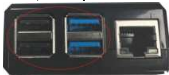
Figure 4 Data ports on Element-D
