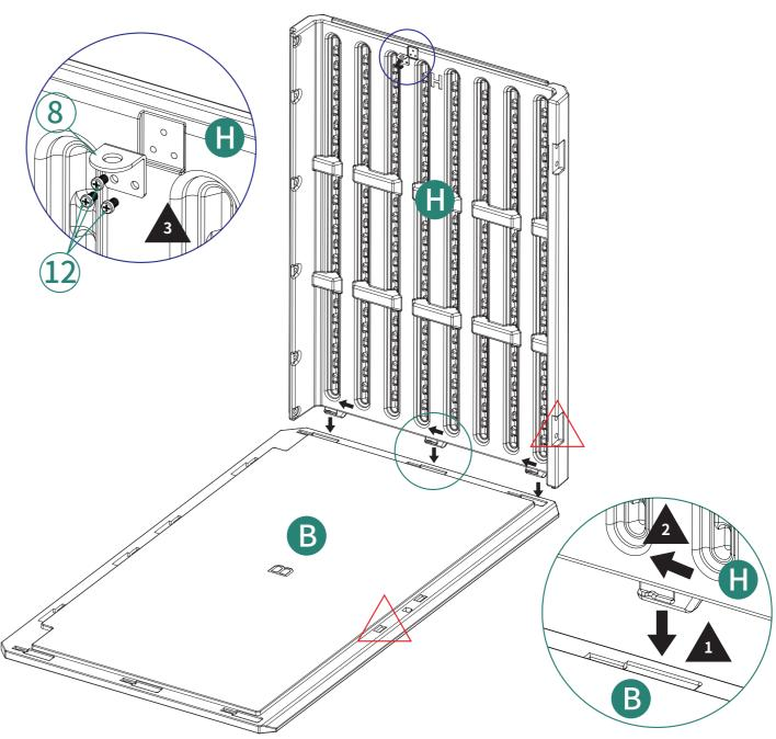
Note: The triangularly marked spots on parts B and H should be on the same side.
