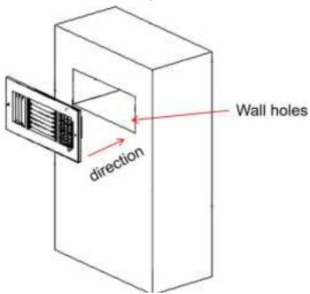
2. Attach the product to the wall through two screws.
