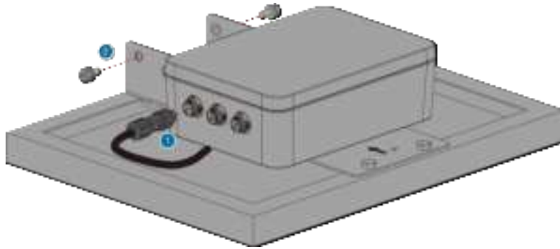
Figure 19: RAK9154 and Solar Panel Connection
