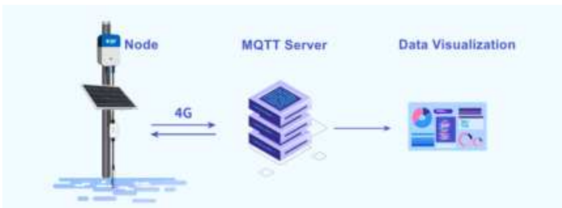
Figure 127: NB-IoT/LTE CAT-M1 application scenario
