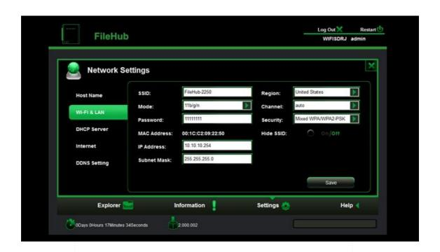
3> DHCP Server: The DHCP or Dynamic Host Configuration Protocol is a network protocol that enables a server to automatically assign an IP address to a computer connected into a network. By default, the DHCP Server option is enabled. And this option can be disabled if needed and the IP address can be manually assigned.
