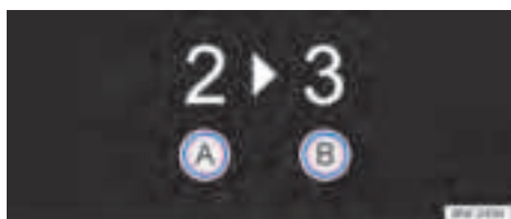
Fig. 96 On the instrument cluster display: gear-change indicator.
