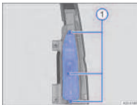
Fig. 178 On the tail lamp cluster: removing the bulb holder.
