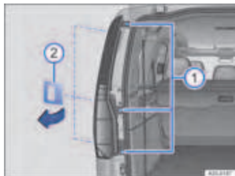
Fig. 176 At the rear left side of the vehicle: removing the tail lamp cluster.
