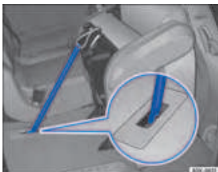
Fig. 67 Second row of seats: secure the seat folded forward with the rod.
