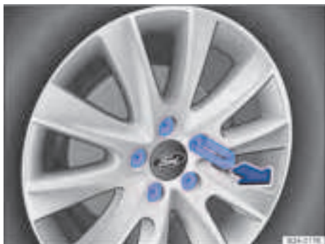
Fig. 214 Removing caps from the wheel bolts with the puller (illustration).
