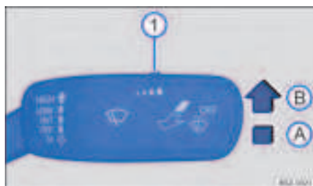
Fig. 84 On the right of the steering column: wiper lever.
