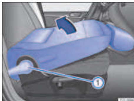
Fig. 62 Front passenger seat: folding the backrest backwards.
