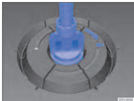
Fig. 224 Connecting the tyre filler hose.
