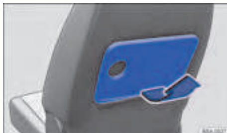
Fig. 126 Front seat: setting up the folding table.
