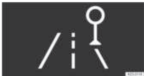
Fig. 25 On the instrument cluster display: Advanced Traffic Sign Display symbol.
