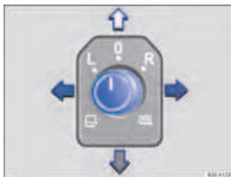
Fig. 87 In the driver door: rotary knob for the exterior mirrors
