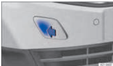
Fig. 189 In the front right bumper: Remove the cover.
