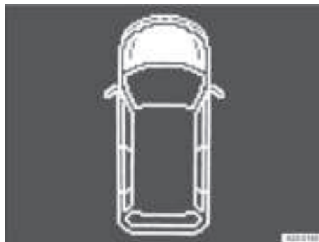
Fig. 197 On the instrument cluster display: the bonnet is open or not closed properly (illustration).
