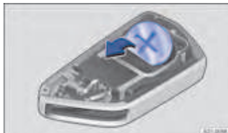
Fig. 52 Vehicle key: changing the button cell.
