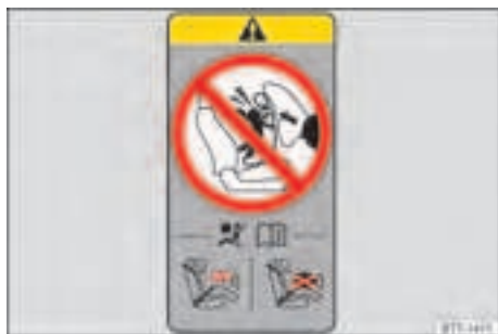
Fig. 39 Illustration: airbag label on the B-pillar.
