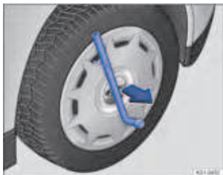
Fig. 213 Pulling off the wheel cover (illustration).
