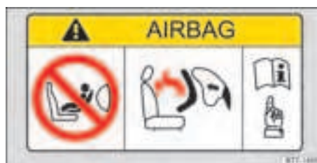
Fig. 38 Illustration: airbag label on the sun visor.
