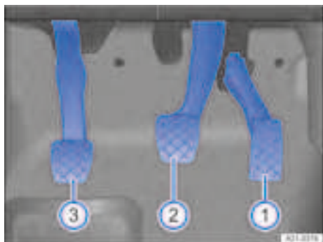
Fig. 90 In the footwell: pedals in vehicles with a manual gearbox.
