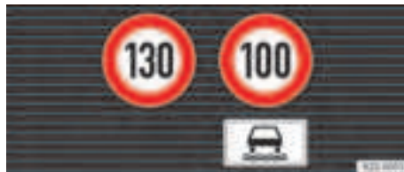
Fig. 26 On the instrument cluster display: displays of Traffic Sign Recognition with detected sub-plate (illustration).
