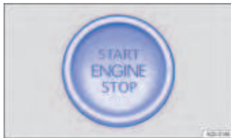
Fig. 91 In the lower section of the centre console: starter button for starting the engine.
