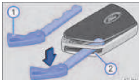
Fig. 51 Vehicle key: opening the cover.
