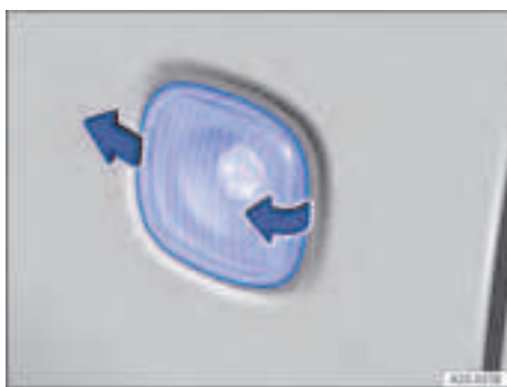
Fig. 174 On the side of the vehicle: removing the direction indicator repeater.
