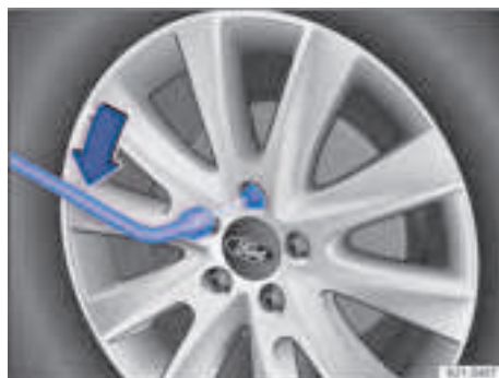
Fig. 216 loosening the wheel bolts.
