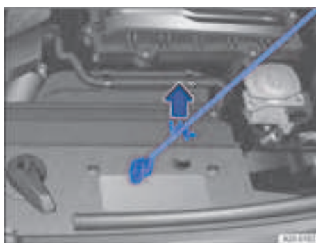
Fig. 195 In the bonnet space: bonnet stay in holder.
