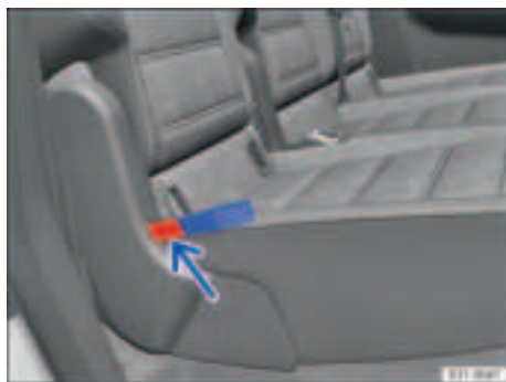
Fig. 65 Second row of seats: marking indicating that the seat backrest is not engaged properly.
