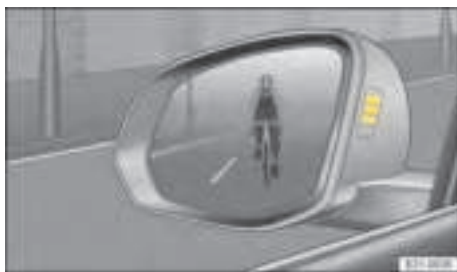
Fig. 113 In the exterior mirror housings: display of the Exit Warning system (illustration).
