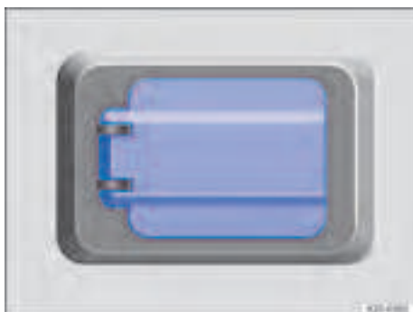
Fig. 129 On the rear centre console or on the partition to the load compartment: 230-volt socket with earthing contact with cover flap (illustration).
