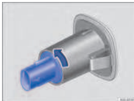
Fig. 175 Replacing the bulb in the direction indicator repeater.
