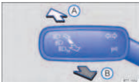
Fig. 79 On the left-hand side of the steering column: direction indicator and high beam lever.
