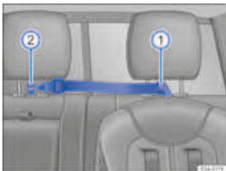
Fig. 45 Attaching the top tether strap (illustration).
