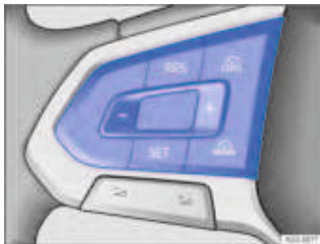
Fig. 102 Left-hand side of the multifunction steering wheel.
