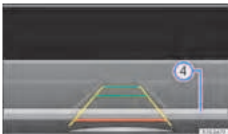
Fig. 117 Infotainment system: aligning vehicle in the parking space.
