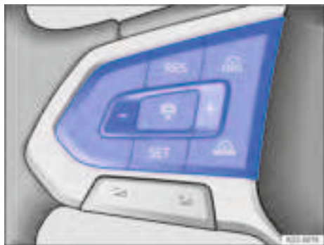
Fig. 110 Left-hand side of the multifunction steering wheel.
