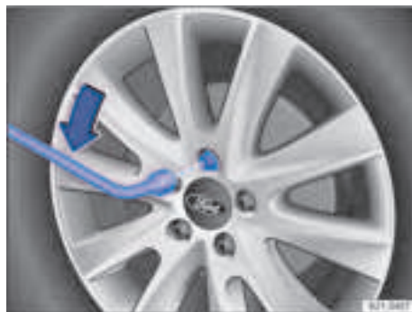
Fig. 220 Unscrew the wheel bolts with the wheel wrench.
