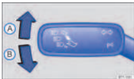
Fig. 80 On the left-hand side of the steering column: direction indicator and high beam lever.
