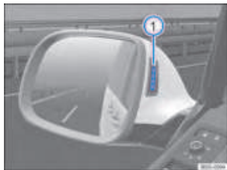
Fig. 111 In the exterior mirror housing: visual displays of Blind Spot Assist.
