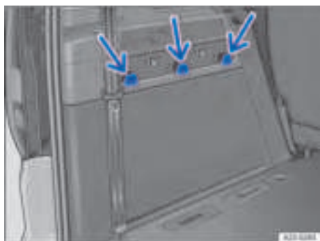
Fig. 142 In the load compartment on the left: bag hook.
