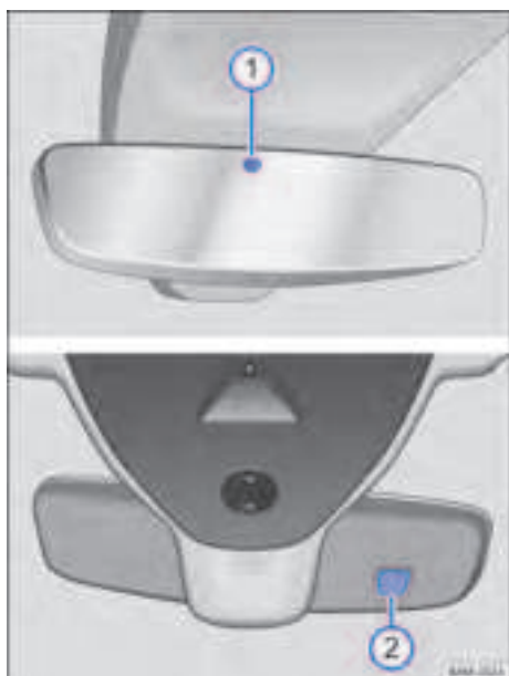
Fig. 85 On the windscreen: automatic anti-dazzle interior mirror.
