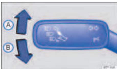
Fig. 77 On the left-hand side of the steering column: direction indicator and high beam lever.
