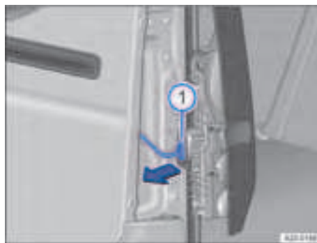
Fig. 177 On the tail lamp cluster: disconnecting the connector.
