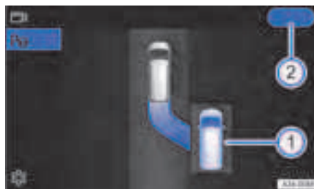
Fig. 120 Infotainment system: procedure for driving out of a parking space (illustration).
