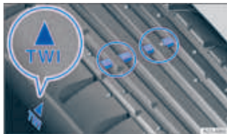
Fig. 210 In the tread grooves: tread wear indicators.
