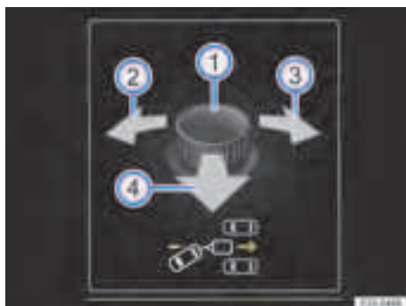
Fig. 121 On the instrument cluster display: adjusting the angle of the trailer using the rotary knob for the exterior mirrors.
