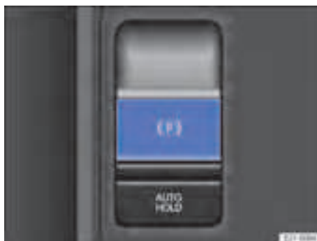
Fig. 112 In the centre console: button for the electric parking brake.
