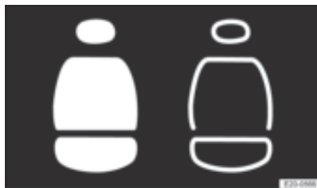
Fig. 28 On the display of the instrument cluster: seat belt warning for the rear seats.
