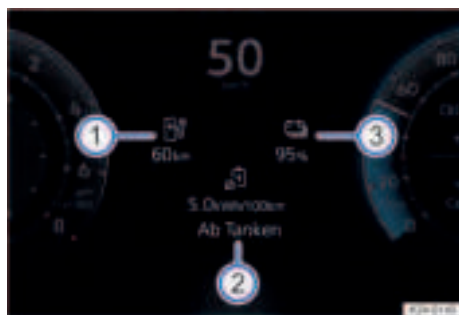
Fig. 15 In the main display area of the digital instrument cluster: charge level and range (illustration).
