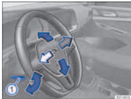
Fig. 57 Below the steering wheel in the steering column trim: lever for adjustment of the steering wheel position.
