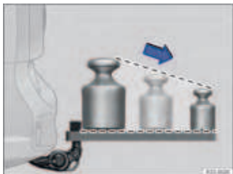
Fig. 145 Recommended weight distribution on the rear carrier system.
