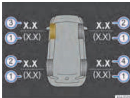
Fig. 211 Display in the Infotainment system: current tyre pressures (illustration).
