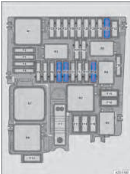
Fig. 180 In the bonnet space: fuse locations.
