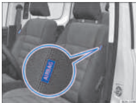
Fig. 34 On the side of the front seat: Location of the side airbag.
