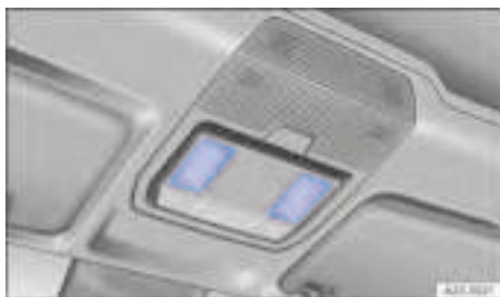
Fig. 81 In the roof console: touch-sensitive reading lights.
