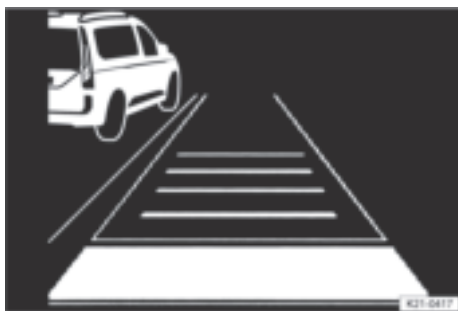
Fig. 103 In the instrument cluster display: slower vehicle detected in the left-hand lane (illustration).
