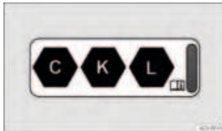
Fig. 157 On the charging socket: sticker for AC charging (C) and DC charging (K, L) with a voltage of up to 920 volts.
