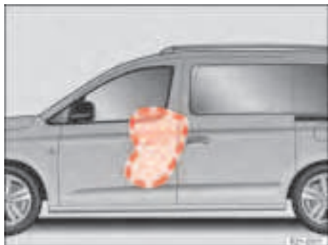
Fig. 33 On the left-hand side of the vehicle: side airbag deployment zone.
