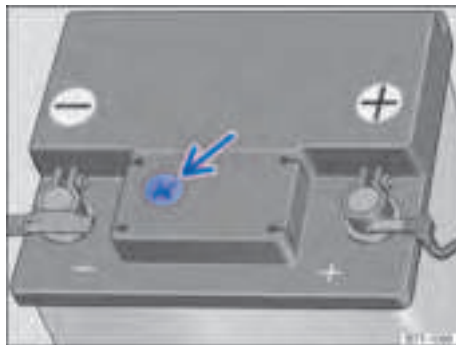
Fig. 206 Battery window on the top of the 12-volt vehicle battery (general guide).
