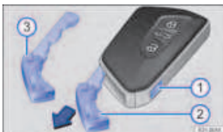
Fig. 49 Vehicle key: releasing the spare key.
