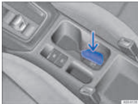
Fig. 92 In the centre console: emergency start function.
