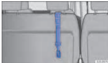
Fig. 44 Middle seat in the second seat row: top tether strap attached in the top tether anchor point (depending on market and equipment).
