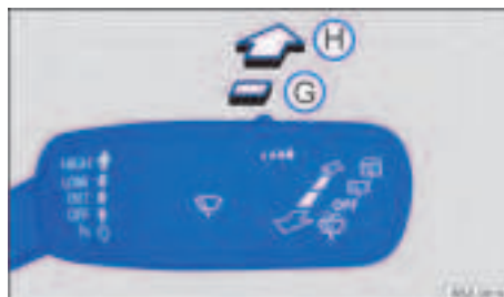
Fig. 83 On the right of the steering column: Operating the rear window wiper.
