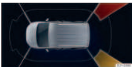
Fig. 124 On the Infotainment system screen: Cross Traffic Alert display.
