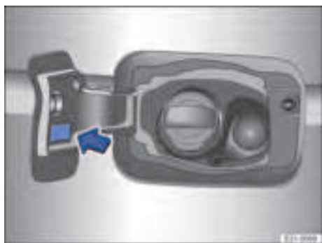
Fig. 148 On the inside of the tank flap: fuel information label (illustration).
