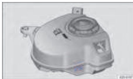
Fig. 204 In the bonnet space: marking on the coolant expansion tank (illustration).
