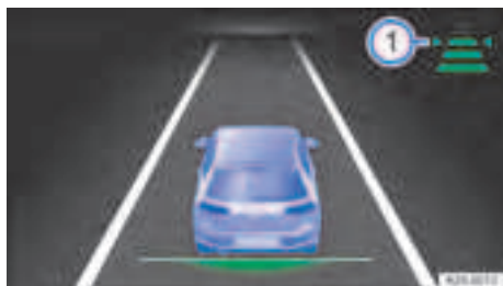
Fig. 106 On the display of the digital instrument cluster: set distance ①, Adaptive Cruise Control is controlling the vehicle (illustration).
