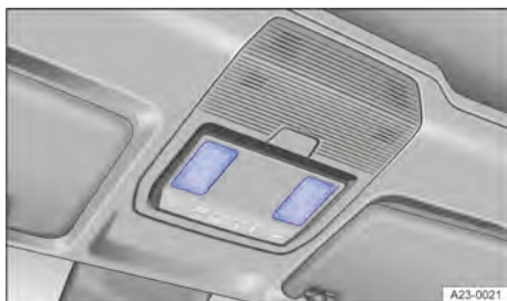
Fig. 81 In the roof console: touch-sensitive reading lights.
