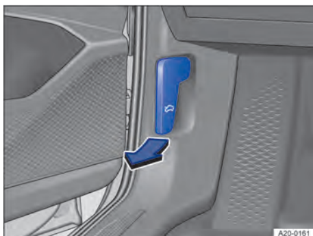
Fig. 193 In the footwell on the left side: bonnet release lever (illustration).
