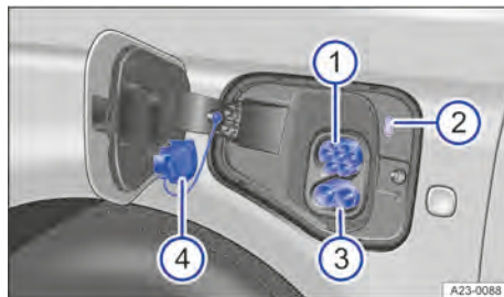
Fig. 158 Behind the charging socket flap at the front left: charging socket.
