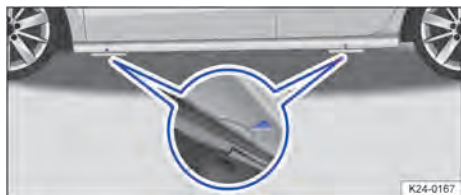
Fig. 217 On the side sill: markings for the jacking points for the jack.
