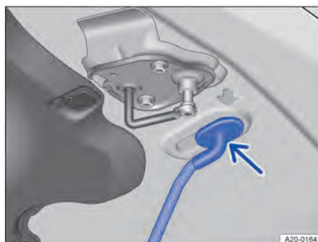
Fig. 196 On the bonnet: holder for bonnet stay.
