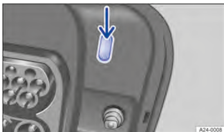
Fig. 160 Behind the charging socket flap: charging process indicator.
