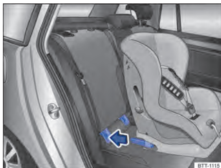
Fig. 41 Illustration: fitting an ISOFIX child seat with the attachment arms.
