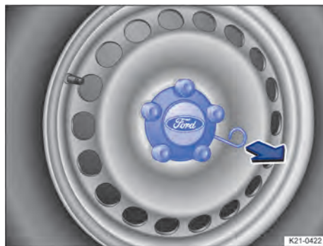
Fig. 212 Pulling off the centre wheel trim (illustration).
