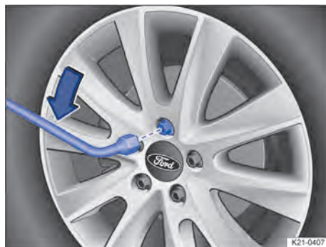
Fig. 216 loosening the wheel bolts.
