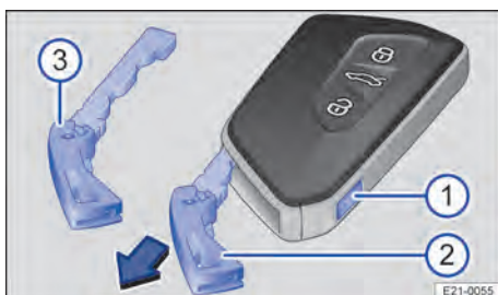
Fig. 49 Vehicle key: releasing the spare key.
