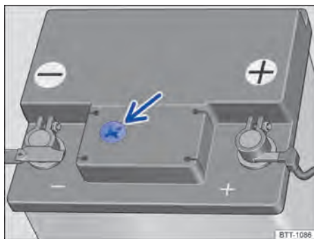
Fig. 206 Battery window on the top of the 12-volt vehicle battery (general guide).
