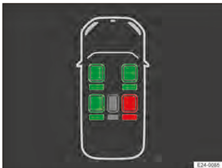
Fig. 29 On the display of the instrument cluster: Seat belt warning system (illustration).
