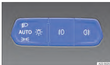
Fig. 78 Next to the steering wheel: touch panel for switching on the exterior lighting.
