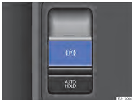
Fig. 112 In the centre console: button for the electric parking brake.
