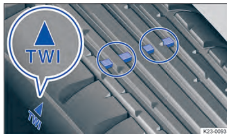
Fig. 210 In the tread grooves: tread wear indicators.
