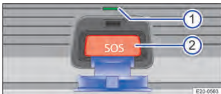
Fig. 48 Control for emergency call: indicator lamp and button for eCall Emergency System.
