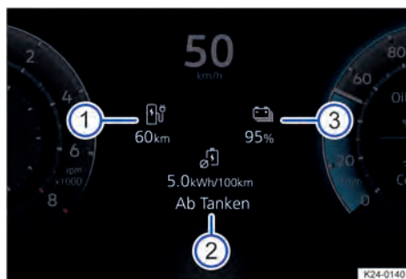
Fig. 15 In the main display area of the digital instrument cluster: charge level and range (illustration).
