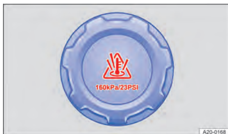
Fig. 203 In the bonnet space: cap of the coolant expansion tank.
