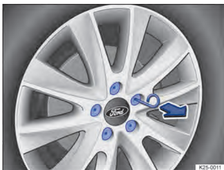
Fig. 215 Removing caps from the wheel bolts with the hook (illustration).
