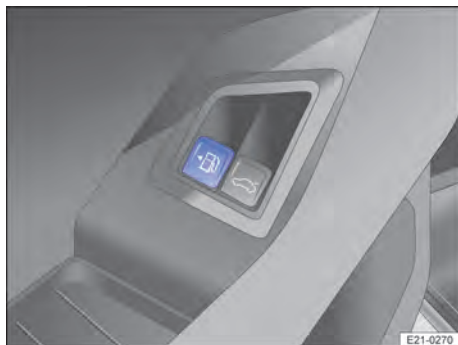
Fig. 153 In the driver door: button for tank flap release (illustration).
