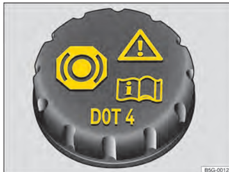
Fig. 205 In the engine compartment: cap on the brake fluid container
