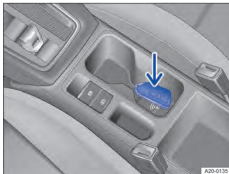
Fig. 92 In the centre console: emergency start function.
