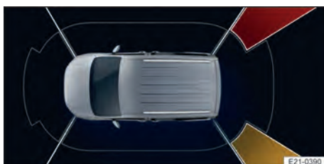
Fig. 124 On the Infotainment system screen: Cross Traffic Alert display.
