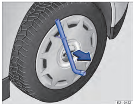
Fig. 213 Pulling off the wheel cover (illustration).
