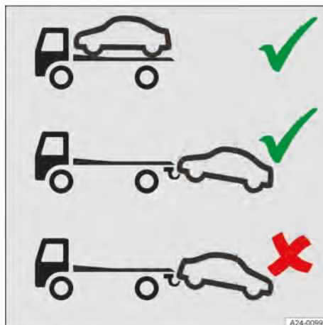
Fig. 188 Transport with a breakdown truck.
