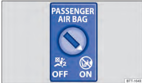
Fig. 30 On the front of the dash panel: key-operated switch for switching the front passenger front airbag on and off.
