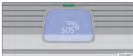
Fig. 47 In the roof console: button for eCall Emergency System (behind button cover) and indicator lamp.
