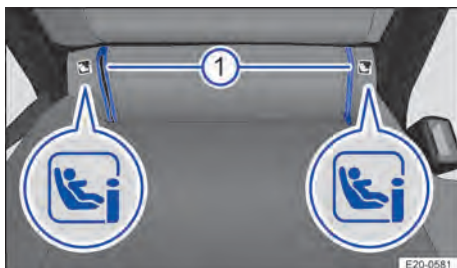
Fig. 40 On the rear seats: different markings identifying the ISOFIX anchor points for child seats.
