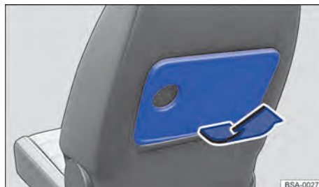
Fig. 126 Front seat: setting up the folding table.
