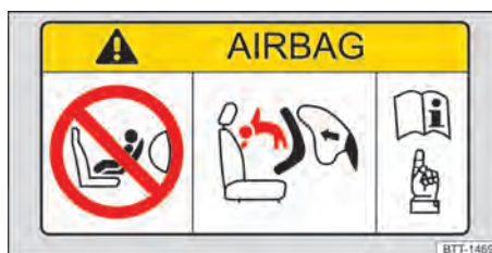
Fig. 38 Illustration: airbag label on the sun visor.
