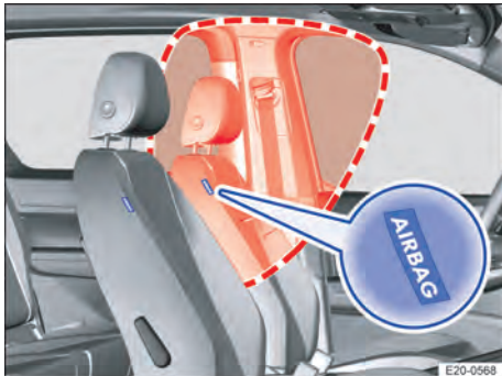
Fig. 37 In the inner backrest cushion on the driver seat: centre airbag. <
