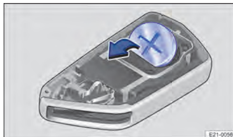
Fig. 52 Vehicle key: changing the button cell.
