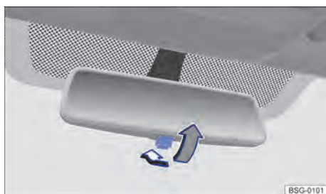
Fig. 86 On the windscreen: manual anti-dazzle interior mirror.
