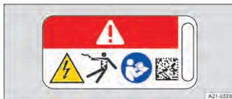
Fig. 154 Warning sign on high-voltage components.
