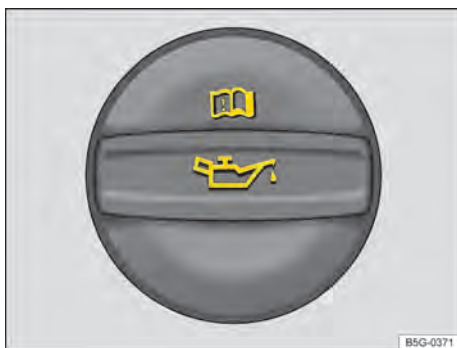
Fig. 199 In the bonnet space: cap of engine oil filler opening (illustration).
