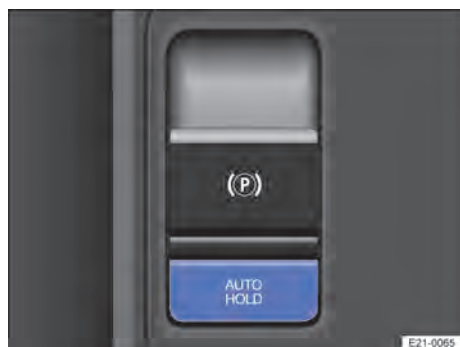
Fig. 114 In the centre console: button for Auto Hold.
