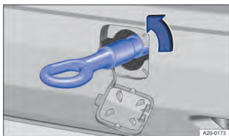
Fig. 192 In the rear bumper on the right: screwing in the towing eye.
