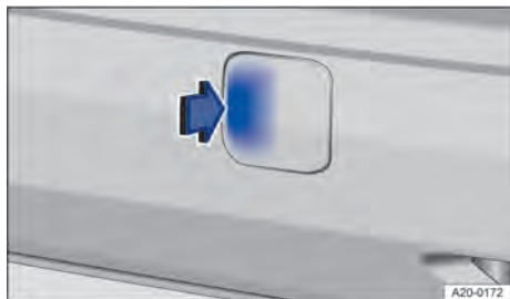
Fig. 191 In the rear bumper on the right: removing the cover.
