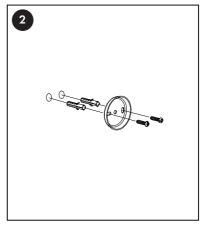
Place the anchors in the drilled holes using a hammer to gently tap them into place. Place the screws through the mounting plate and thread them into the anchors.
