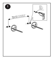
Use a measuring tape and pencil to mark the area where the item will be installed. Ensure the markings are level.
