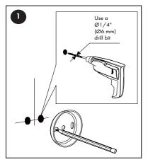
Mark the area where the item will be installed. Use a level to make sure that the mounting hardware is level. Drill  $\varnothing 1/4$ " ( $\varnothing 6$  mm) holes for the mounting hardware.
