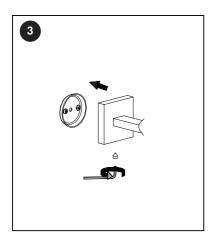
Place the item onto the mounting plate and use an Allen wrench to tighten the set screw, securing the item to the mounting plate. Ensure that the item is not upside down.
