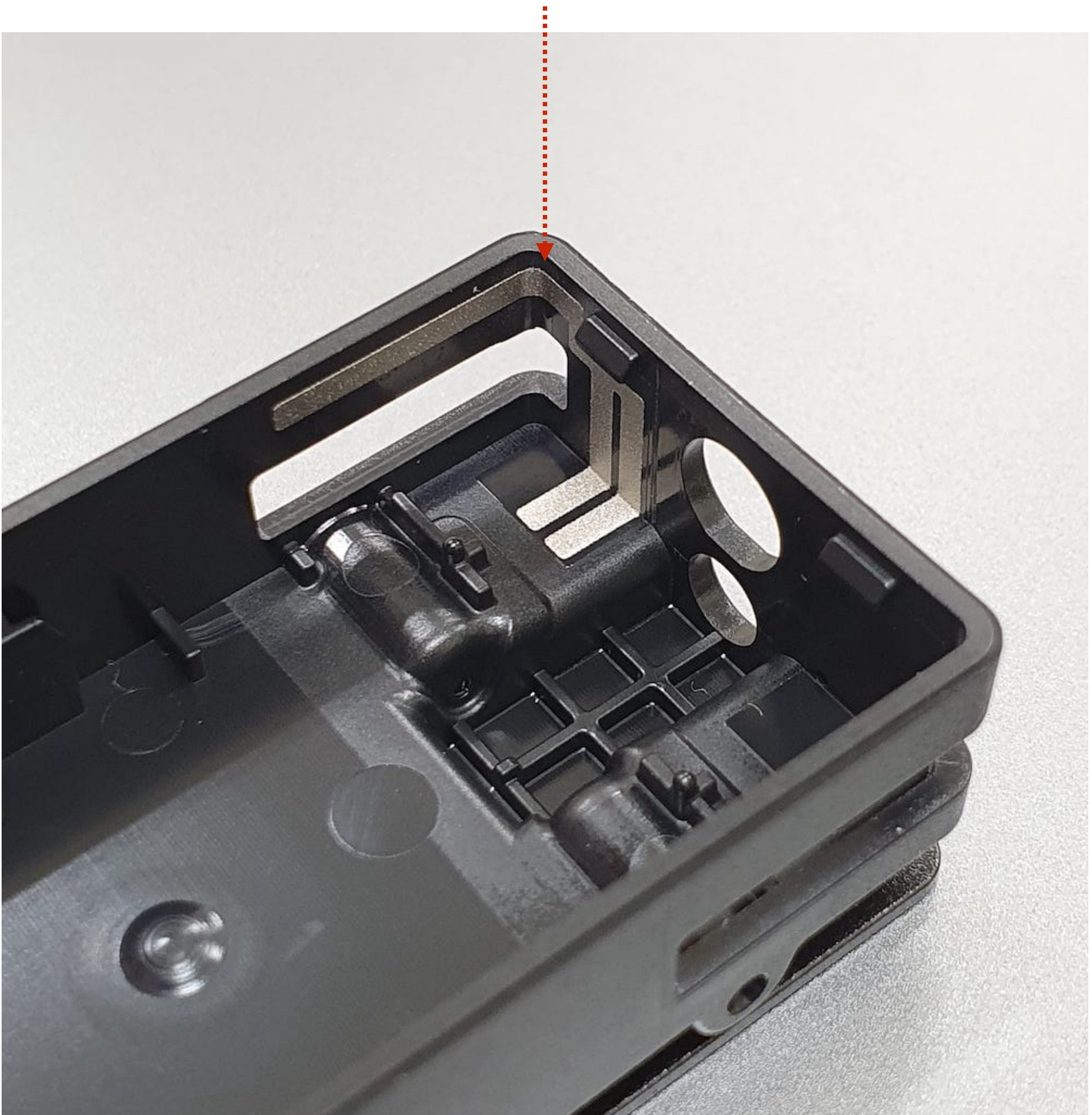
3 Dimensional LDS (Laser Direct Structuring) Antenna
