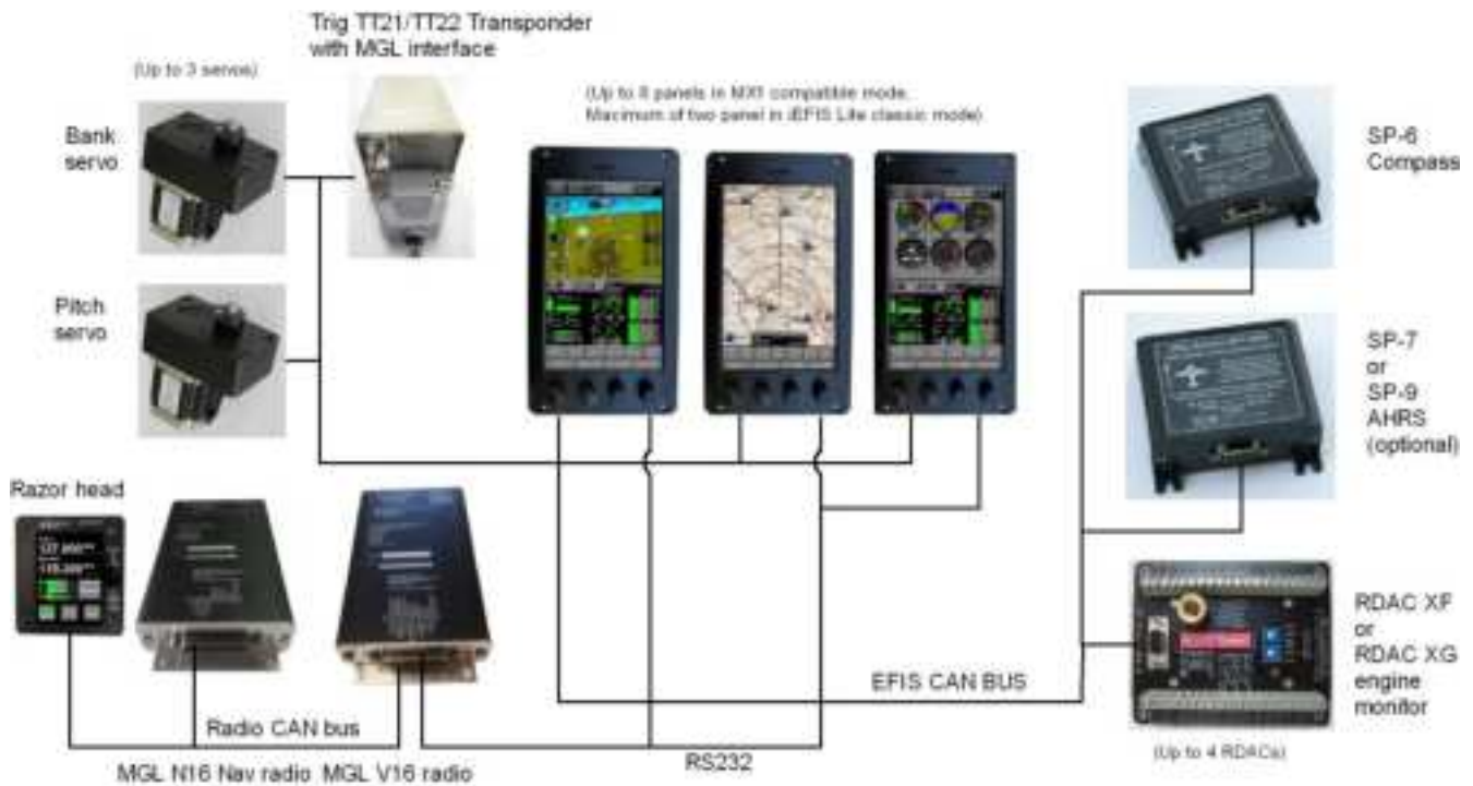
Example iEFIS G4 MX2 Lite system layout for a three panel solution, showing main communications bus connections.
