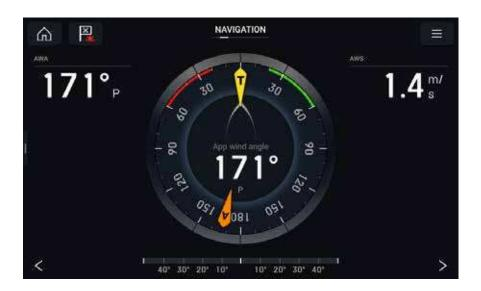
• If ,for some reason, you don't see a zero data in your dashboard, it means that the NCP High-End is connected but it is not receiving data from the wind meter. In this case, please double check the wind meters' connection. If you see nothing (please see picture below), it means the NCP High-End is not well connected. Please, double check the connection. If the issue persists please contact us at sales@calypsoinstruments.com.
