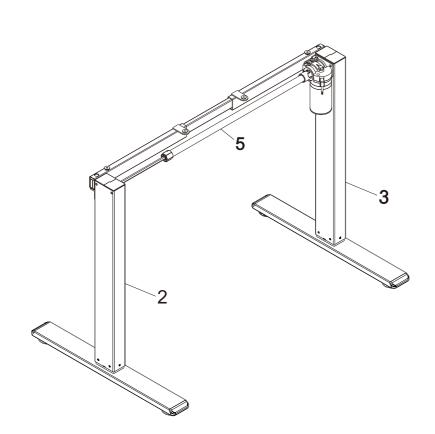
Connect support beam (6) with columns (2,3) by screw F, then tighten screw C in holes on side beam by 5x5 wrench A.
