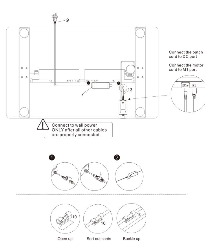
The cable tie (10) can be used to fasten the cables to the desktop.
