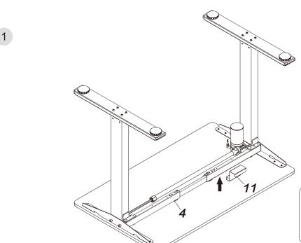
Note: the holes in the adapter holder (11) are not for screws.
