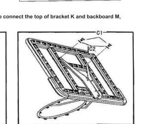
As shown in the figure, use screws F1,F2,F3 to fix top pole W in the middle of bracket K.
