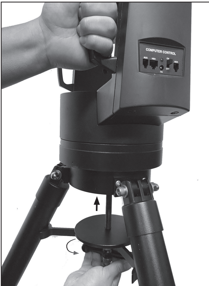
Fig. 5: Place telescope on top of tripod carefully and secure in place.
