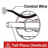
The Tail Piece that goes through the door and connects the lock (See Diagram) MUST be in the VERTICAL position (Up and Dowr during installation
