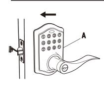
Check that the rubber gasket is secured on the exterior assembly. Insert the exterior assembly onto the door with the tailpiece going through the deadbolt latch set in the **VERTICAL POSITION**. Route the control wire through the door under the deadbolt
