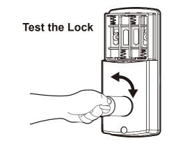
Lock/Unlock: using the knob to make sure the latch is retracting easily. If not, go back to step 3.
