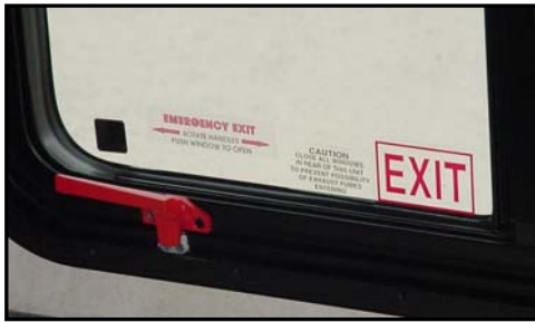
Figure 13-2. Emergency Exit Window
