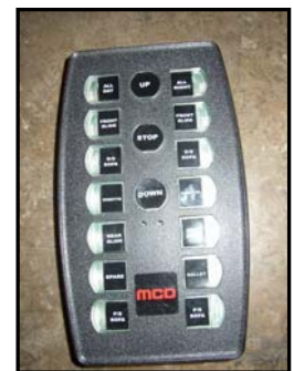
Figure 10-4. Control for Living Area Power Shades
