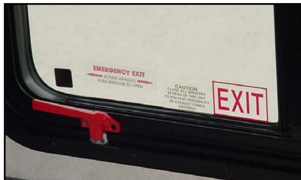
Figure 2-9. Emergency Exit Window
