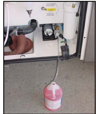
Figure 14-17. Winterizing the Water System
