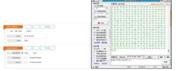
(7) After successful configuration, Net Assistwill receive data from the gateway. Can be parsed based on Bluetooth gateway data protocol;
