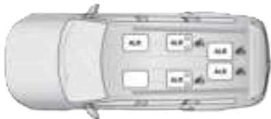
Captain's Chairs Second Row (6 Passenger) Automatic Locking Retractor (ALR) Locations
