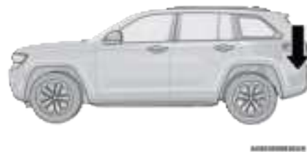
Sensor Location (Left Side Shown)
