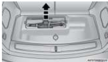
Jack Removal (Equipped Without Air Suspension)
