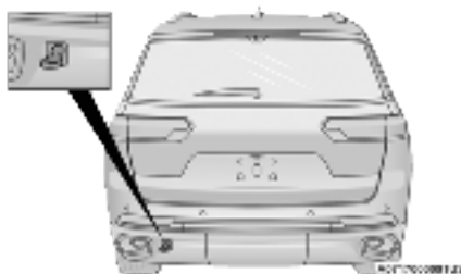
Rear Tow Eye Installed
