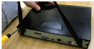
Replace the cover and fasten screws
