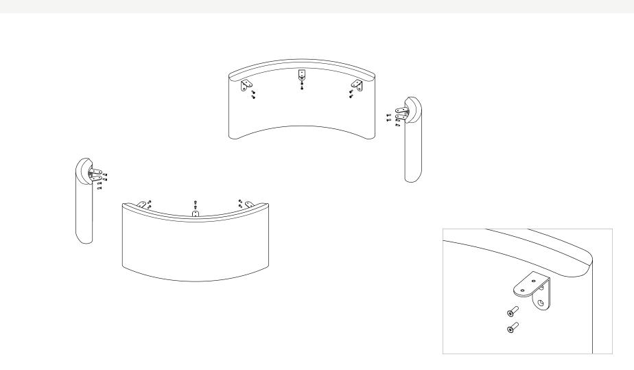
Rest the undermount on the ground with the underside facing up, then place the legs on top of it, ensuring the holes on the corner brackets align with the holes on the undermount. Insert two flat head screws into each corner bracket and tighten them using the Allen wrench.
