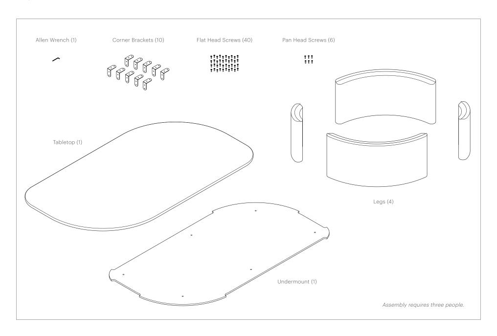
Keeping the tabletop in its crate, place it on the floor with the underside facing up. Use the Allen wrench to remove the pan head screws on the bottom of the undermount, then separate the undermount from the tabletop.
