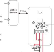
Step 1: Short press "reset" button 4 times (Or reset power of the device from master breaker) to start TouchLink Commissioning, 180 seconds timeout, repeat this step.
