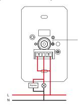
Step 1: Short press "Reset." button 3 times (Or reset power of the device (initiator node) 3 times from master breaker) to start Find and Bind mode (connected light flashes slowly) to find and bind target node, 180 seconds timeout, repeat this step.
