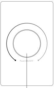
Rotary knob, short press to turn on/off, rotate clockwise to increase brightness, rotate counterclockwise to decrease brightness
