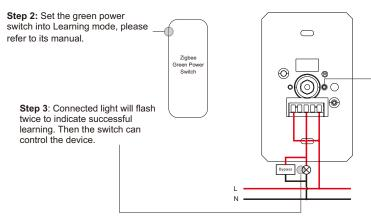
Step 1: Short press "Reset." button 4 times (Or reset power of the device 4 times from master breaker) to start Learning to GP switch mode (connected light flashes twice), 180 seconds timeout, repeat this step.
