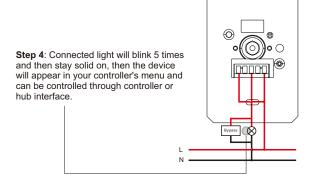
Step 3: power on the device, it will be set into network pairing mode (connected light flashes twice slowly), the network pairing mode will last until the device is added to a zigbee network.
