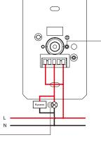
Step 1: Short press "Reset." key for 5 times continuously or reset power of the device from master breaker for 5 times continuously if the "reset" key is not accessible.
