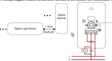
Step 1: Short press "Reset." button 4 times (Or reset power of the device 4 times from master breaker) to enable the device to setup a zigbee network (connected light flashes twice) to discover and add other devices, 180 seconds timeout, repeat this step.
