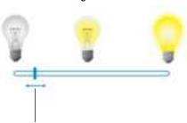
Step 1: adjust the brightness of connected load to 100%.
