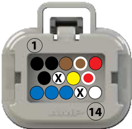
End of 14-pin ABS power harness
