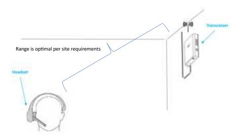
2. If the system audio and range tests are optimal, proceed to tighten down the screws on the Transceiver mounting plate by sliding the Transceiver out and sliding it back on once the screws are tightened. Otherwise repeat the steps above.
