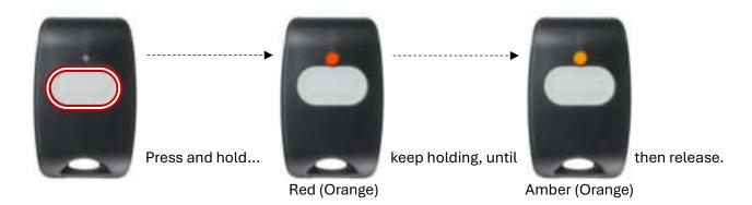
Fech Tip: If the LED flashes only once after holding for 10 seconds, or if it flashes multiple times the keyfob may have been enrolled into another panel.
