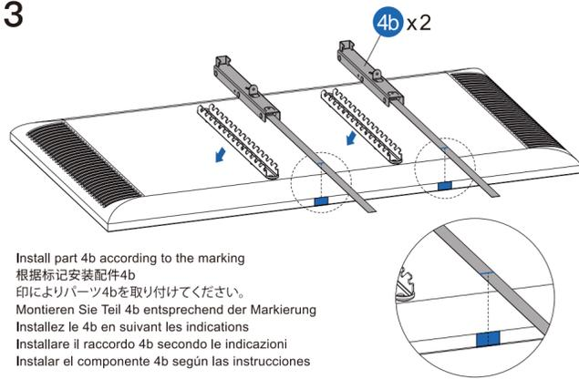
Install part 4b according to the marking
