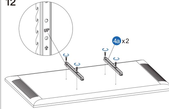
Select appropriate screws from M-A to M-G and install part #4a on the four screw holes on the back of the TV. The back of the TV is flat, and the A1 installation method without gasket can be used; if the back is uneven, A2 installation method with washers (M-H to M-J) can be used, and thick washers can be superimposed according to the situation.
