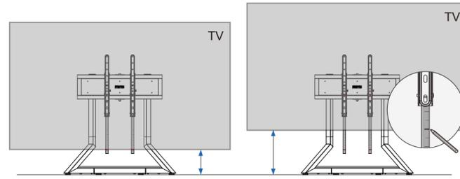
The adjustable range of the distance from the bottom of the TV to the ground is marked on the part 4, so that you can choose the appropriate height. You can choose the height, make a mark on the ruler, and then disassemble and install the part 4 to the back of the TV.
