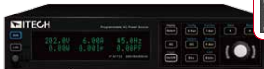
Loading 40 order harmonic components
