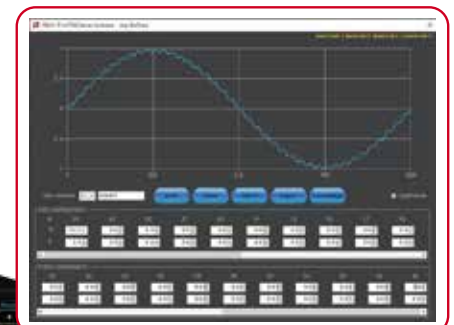
Loading 40 order harmonic components
