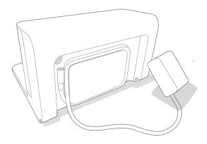
Plug the power cord into the wall. Wrap the cord back so it won't get in the way of the robot as it comes and goes.
