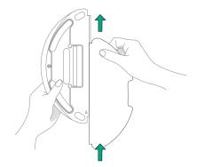
2 Fill the tank with water by opening tank lid, filling the tank with water, and reattaching the lid.
