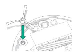
IMPORTANT: It is recommended to replace the edge-sweeping brush every 3-6 months for an optimal cleaning effect.
