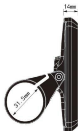
Fig. 3-4 Side View of Display 80C Dimensions
