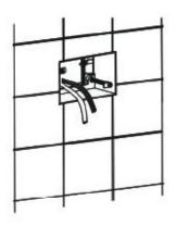
Measure the depth of the flush plate and create a cavity in the wall equal to the depth of the flush plate. Pull the pipes for installation through the cavity and thread them through the back of the base. Insert the base into the wall and Screw the fixing arms (supplied) into position. The rods may need cutting down depending on the thickness of the finished wall/surface.
