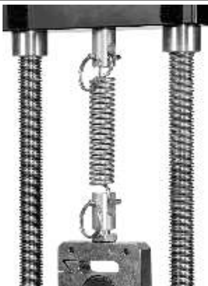
Figure 8: A spring secured in place using the Clevis Grip.
