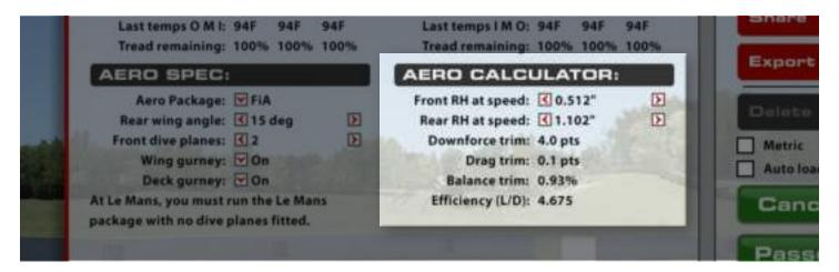
The Aero Calculator is a tool provided to aid in understanding the shift in aerodynamic balance associated with adjustment of the rear wing setting and front and rear ride heights. It is important to note that the values for front and rear ride height displayed here DO NOT result in any mechanical changes to the car itself, however, changes to the rear wing angle here WILL be applied to the car. This calculator is a reference tool ONLY.
