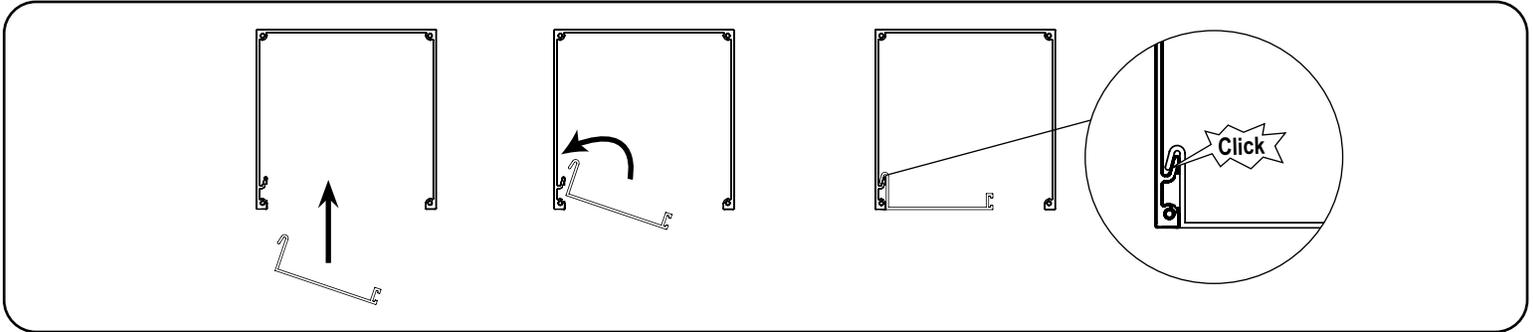
**To install**, insert the bottom closure into pocket on an angle, hook onto the front side of the pocket. Once it is aligned, carefully allow front of bottom closure to drop in place.
