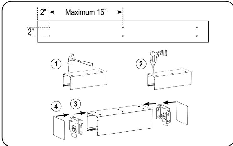
Using a pencil, mark the screw hole locations. Use a center punch on the marked locations. Pre-drill mounting screw using a 1/8" drill bit. Insert Bracket into pocket (may need mallet to gently tap bracket into place) until flush with end of pocket. Secure the end plates into the pocket using the provided screws.
