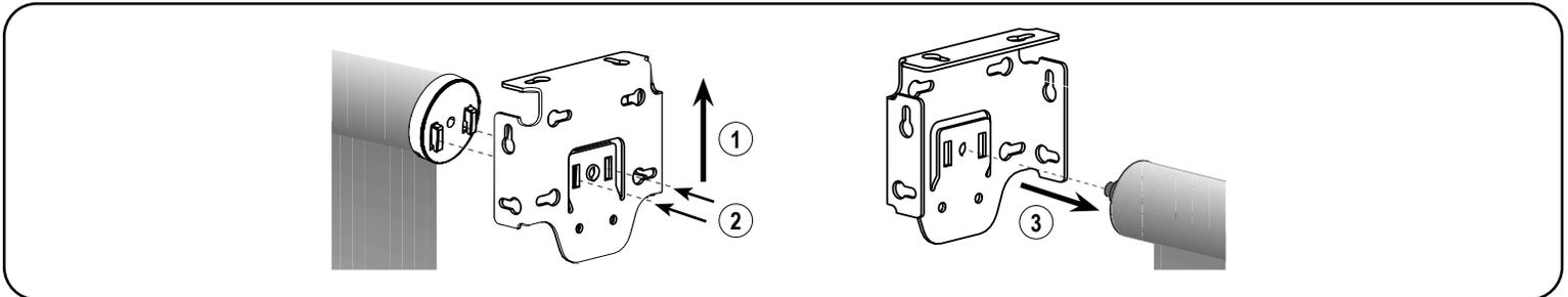
First, follow steps to remove the bottom closure. Then, gently lift the control unit (hooks end) to disengage, until the hooks touch the top part of the bracket slot. Pull the shade towards the spring loaded pin end until the hooks are completely out of the bracket slots. Finally, remove the spring loaded pin end from the Idler bracket.
