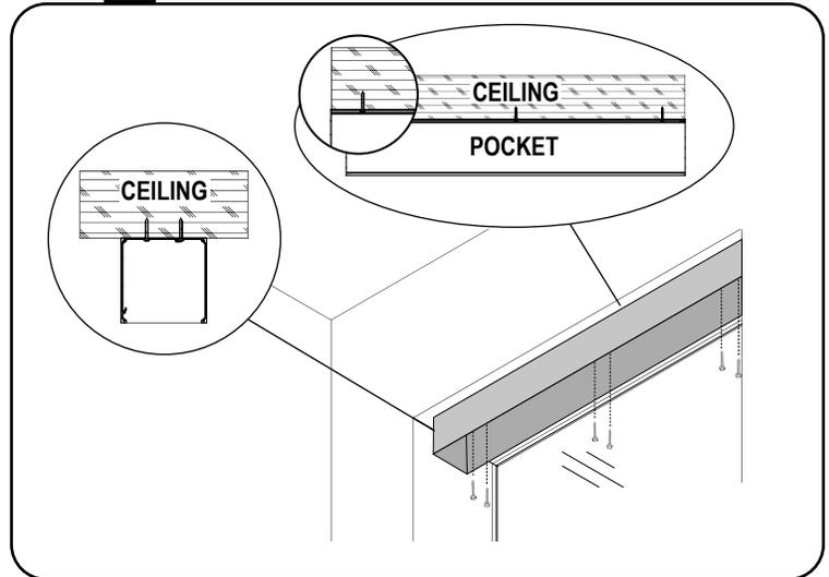
Respecting the pre-drilled holes, mount pocket to ceiling using the appropriate mounting screws. **Important:** Secure bracket to pocket/ceiling with supplied mounting screws.
