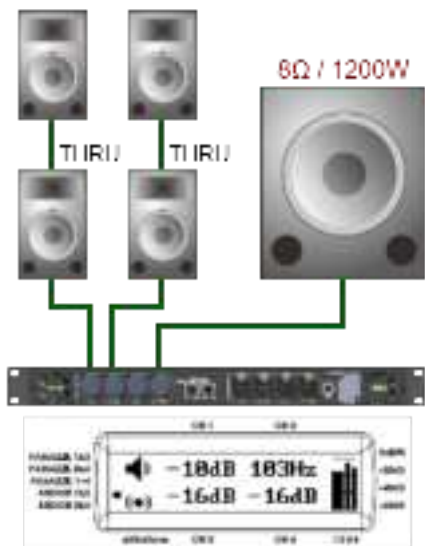
x3 configuration with mix of a bridged output on the 1st pair of outputs. estimated max. output: 1200W + 600Wx2
