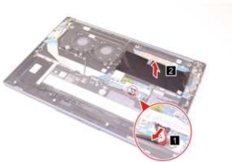
Figure 20. Disconnect the battery pack cable and peel off the mylar
