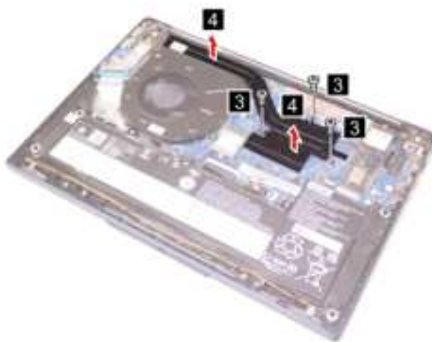
Figure 23. Loosen three screws and remove the heat sink
