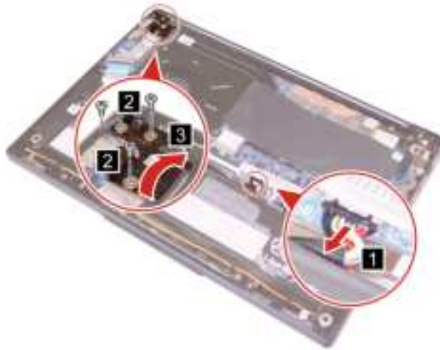
Figure 24. Disconnect the battery pack cable, remove three screws and open the hinge.
