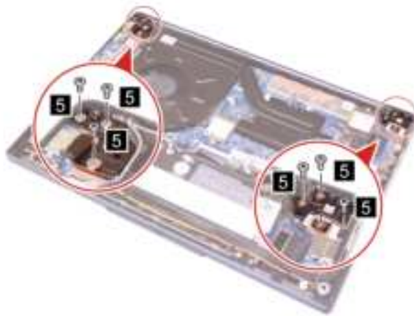
Figure 46. Remove six screws and rotate the LCD unit
