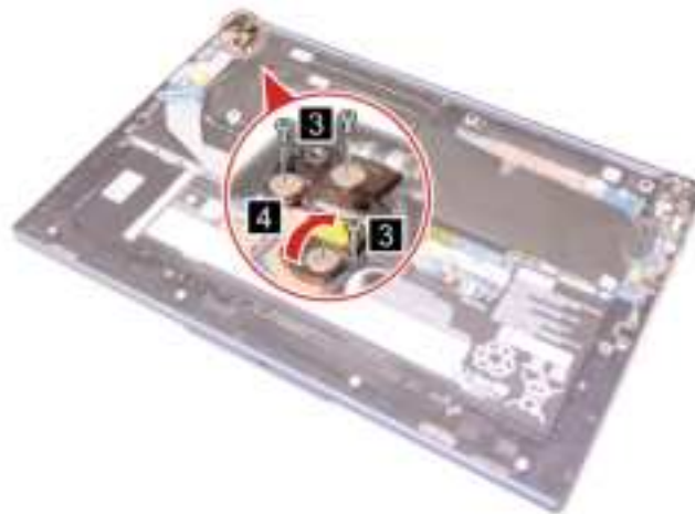
Figure 27. Remove two screws and open the hinge
