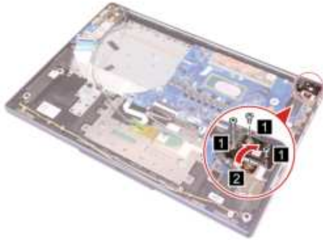
Figure 32. Remove three screws and open the hinge
