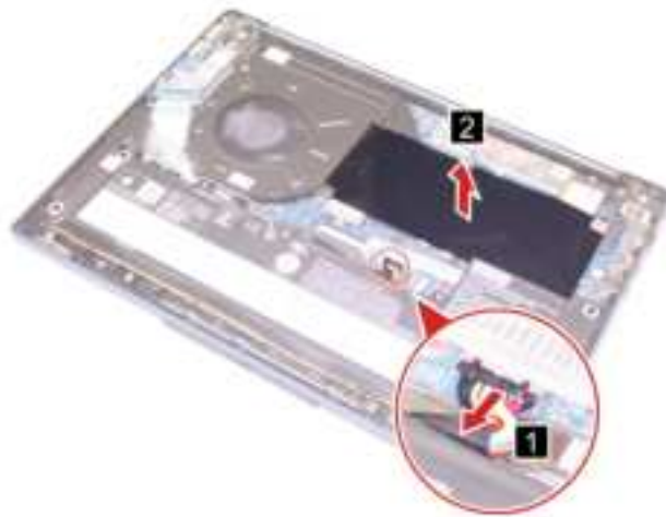
Figure 17. Disconnect the battery pack cable and peel off the mylar
