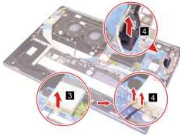
Figure 49. Disconnect antennas and EDP cable
