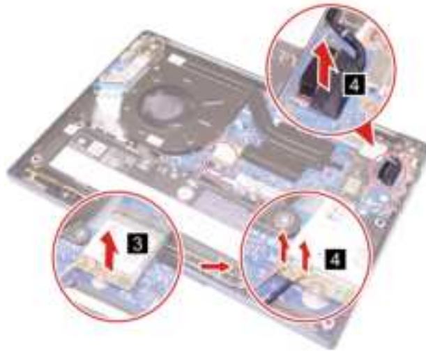
Figure 45. Disconnect antennas and EDP cable from the system board
