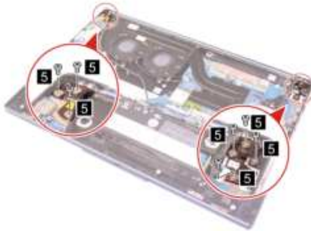
Figure 50. Remove six screws and rotate the LCD unit
