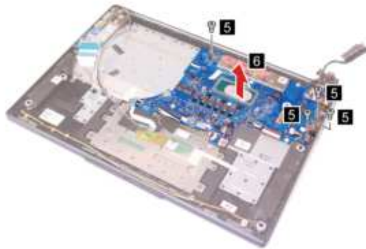
Figure 34. Remove four screws and the system board with I/O board cable
