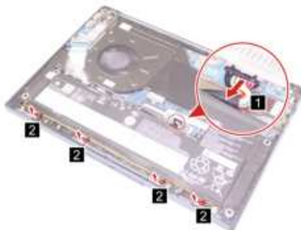
Figure 5. Disconnect the battery pack cable and take the speaker cable out of the cable guide
