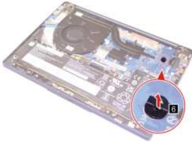
Figure 10. Remove the 2242 solid-state drive holder
