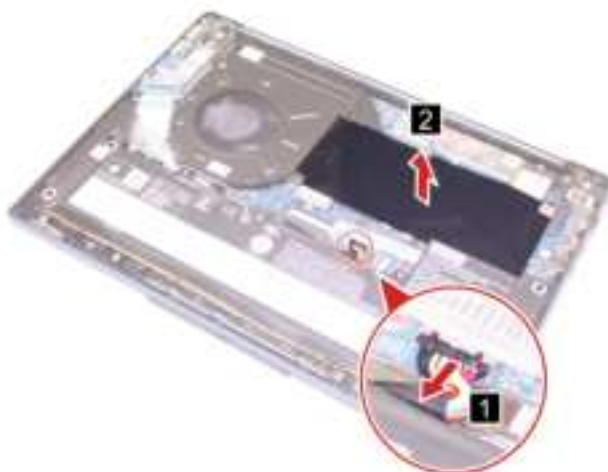
Figure 22. Disconnect the battery pack cable and peel off the mylar
