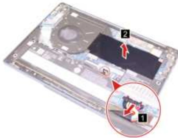
Figure 14. Disconnect the battery pack cable and peel off the system board mylar
