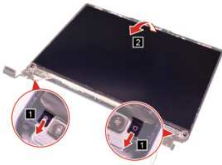
Figure 56. Pull out the removable tapes and lift the LCD panel.
