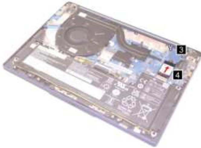
Figure 8. Remove the 2242 solid-state drive
