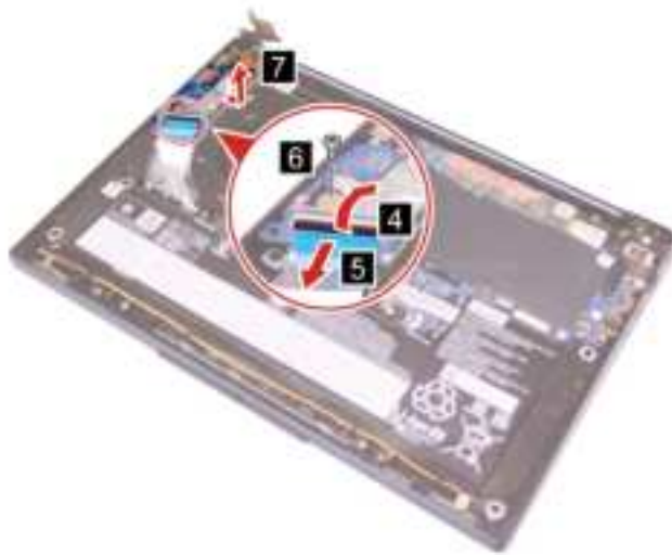
Figure 25. Disconnect the I/O board cable, remove one screw and the I/O board
