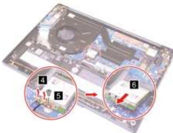
Figure 16. Disconnect the wireless antennas and remove one screw and the Wi-Fi card
