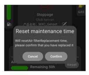
After replacing the components, click the button and confirm in the pop-up window to manually reset the maintenance time.
