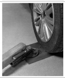
The DRAW ALIGNER PRO has a rotating pole to change the pull angle to suit the pulling situation.
