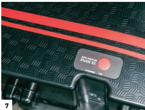
[7] Once the Auto Position button on the side of the housing is pushed, the voice commands guide the user through the set-up process. [8] A logical place to mount the breakaway switch was on the topside of the safety chain loop, attached to the baseplate. A coiled cable [9] is routed from the switch to the hitch receiver on the motorhome when towing.
