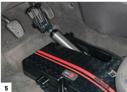
[3] A seat floor pan with a lip in the back is needed to position the RViBrake3 properly. If the dinghy vehicle has a flat floor pan, the provided stop plate [4] can be installed. [5] Low-profile housing makes it simple to position on the floor pan in the test Ford Fiesta. Well-designed claw [6] attaches to the brake pedal without the use of tools.
