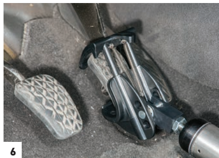
[3] A seat floor pan with a lip in the back is needed to position the RViBrake3 properly. If the dinghy vehicle has a flat floor pan, the provided stop plate [4] can be installed. [5] Low-profile housing makes it simple to position on the floor pan in the test Ford Fiesta. Well-designed claw [6] attaches to the brake pedal without the use of tools.
