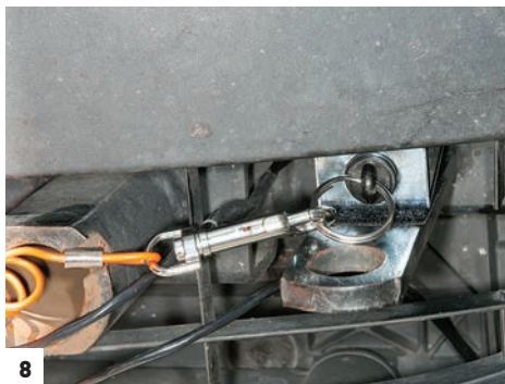
[7] Once the Auto Position button on the side of the housing is pushed, the voice commands guide the user through the set-up process. [8] A logical place to mount the breakaway switch was on the topside of the safety chain loop, attached to the baseplate. A coiled cable [9] is routed from the switch to the hitch receiver on the motorhome when towing.
