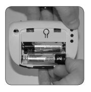
3 STILL HOLDING the chime selection button, switch the power back on by INSERTING THE BATTERIES.
