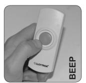
**PRESS** the bell push. An audible beep will be heard again from the receiver. The receiver is now being programmed.
