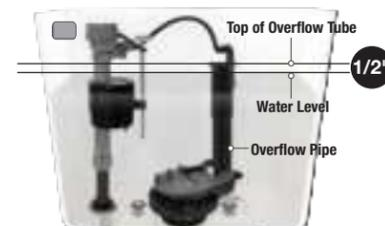
\* Overtightening may damage fill valve, potentially causing flooding. Make sure the float cup does not touch the tank walls or tank lever and flush valve.
