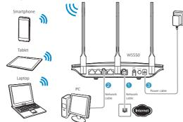
2 Check the **SSID** on the label attached to the bottom of the WS550 (unencrypted by default), and then wirelessly connect your phone to the WS550's Wi-Fi network.
